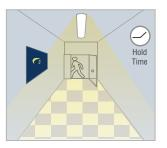
After the last detection the light will be dimmed to the stand-by dimming level (10, 20, 30 or 50%) after hold time
