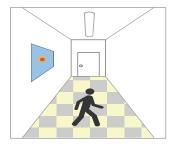
With sufficient daylight, even with the motion sensor detected, light remains OFF
