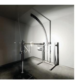
Photometry defines the measurement and distribution of light output to help lighting professionals select products and options that are most appropriate to their requirements. Photometric data of our entire products range is measured in a lighting laboratory with a digital goniophotometer, ensuring a correct and realistic lighting design
