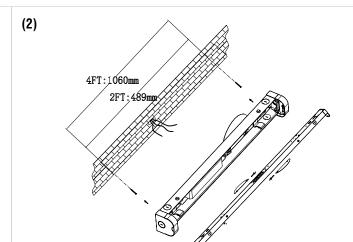
Install sheet metal to cover the junction box, semi-lock the screws into wall.
