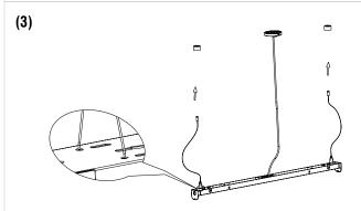
Lock the steel rope into the fixture bracket, fix the end of the steel rope into the holder, then thread AC wire through the bracket.
