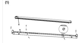
Take out the lamp, press the snap-on button and remove the cover.
