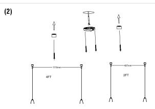
Fasten the holder and self-lock device on the ceiling.
