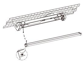
Adjust desired CCT using the slider switch, connect DC plug, then buckle the fixture cover.
