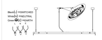
Connect AC wires accordingly
