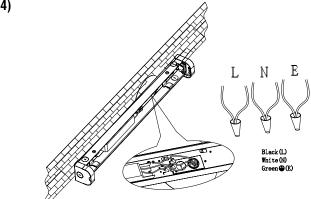
Connect AC wires accordingly.
