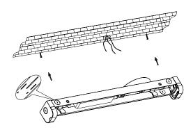
Align and hang the mounting holes of the fixture bracket with the screws on the wall, then tighten the screws again.
