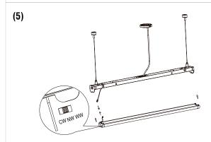
Adjust desired CCT using the slider switch, connect DC plug, then buckle the fixture cover.
