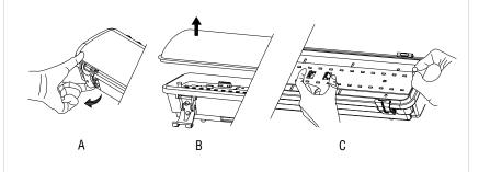
1 Loosen cable gland tightening nut, insert the cable through the gland
