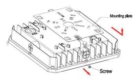
3. Hang the lamp on the ring so as to connect wires with terminal caps
