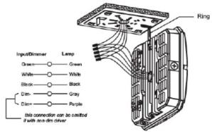
4. Secure the screws, installation completed
