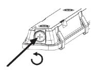
3. Insert the cable through the waterproof connector and terminate wiring into the terminal block. Ensure L, N, Ground wires are connected correctly
