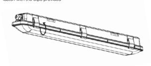
2. Fasten on the supplied waterproof connector clockwise
