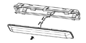
6. Connect purple dim + / gray dim - to the 0-10V dimming wires
